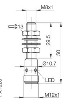
**Inductive Sensors** BES M08ME1-GSC20B-S04G M8x1x50 normally-open Sn=2mm shielded
